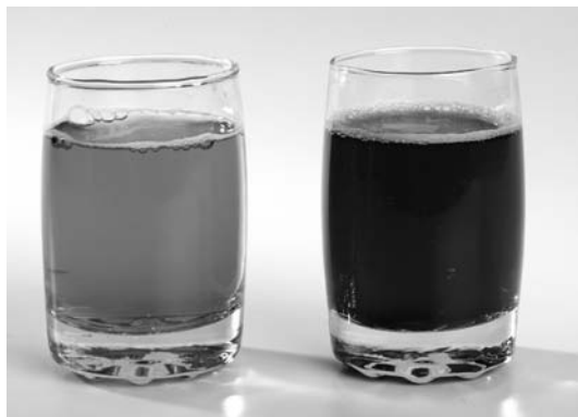
Figure 3 You can make a concentrated solution by adding a lot of solute. You can make a dilute solution by adding less solute to the same volume of solvent.
